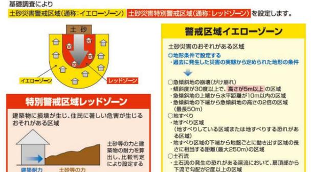
Diagrams and descriptions for 急傾斜地の崩壊 (Slope failure), 地すべり (Landslide), and 土石流 (Debris flow).
